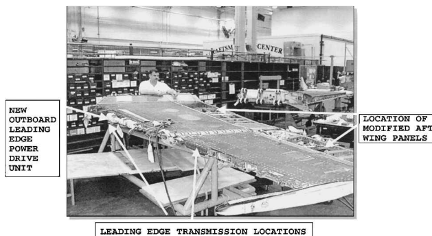
Fig. 5 Wing modification/leading-edge flap drive location.
